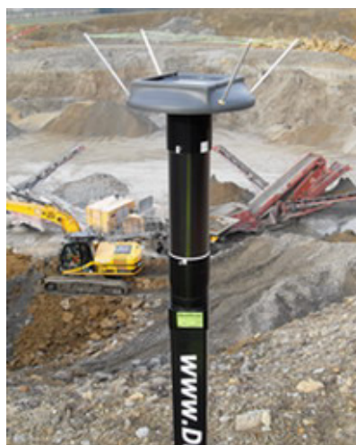
Fig 1 – Sticky Pad Dust Sampler
