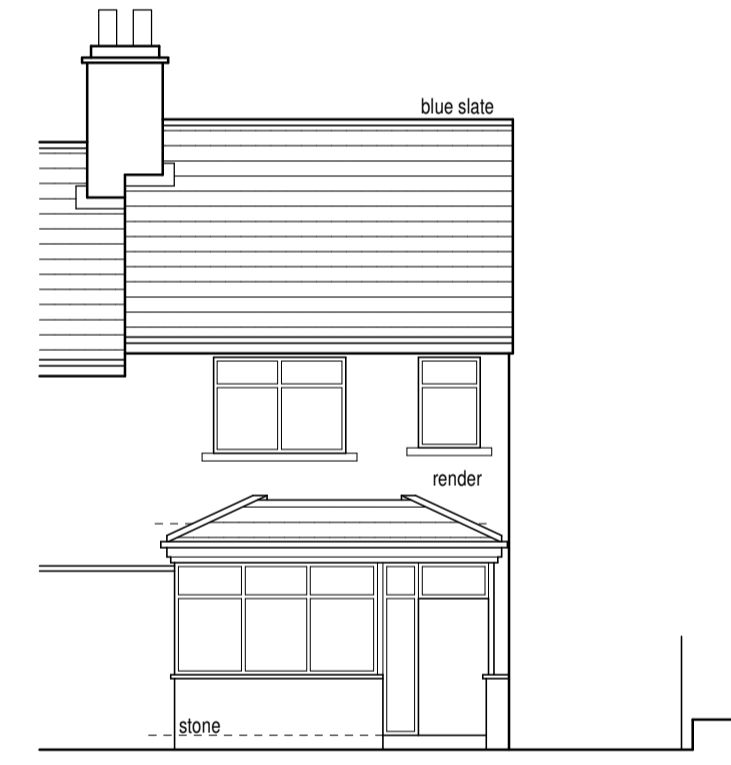
Existing front elevation (1:100)
