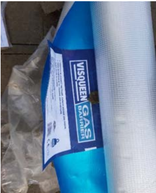
Gas Barrier Membrane: Visqueen Gas Barrier
