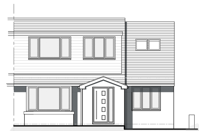
Proposed North East Facing Front Elevation Scale 1:100
