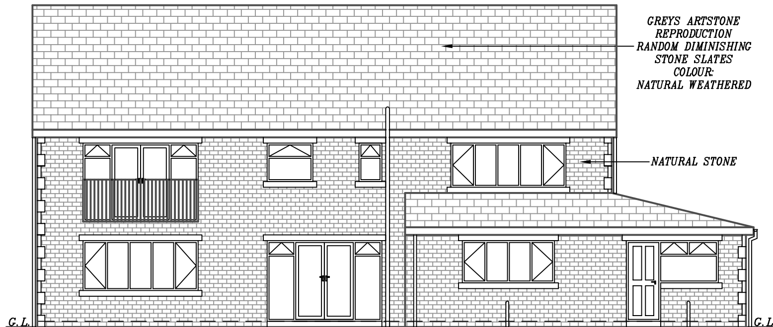
PROPOSED REAR ELEVATION (24 PROSPECT TERR)
