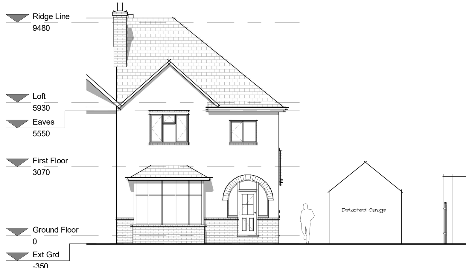
Front Elevation (East Facing) 1 : 100
