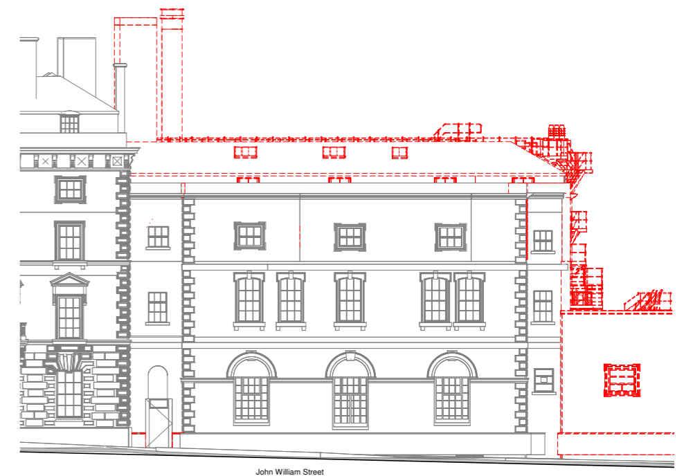
DRAWING EXTRACT 4 : John William Street elevation showing extent of proposed demolition for Block C.
