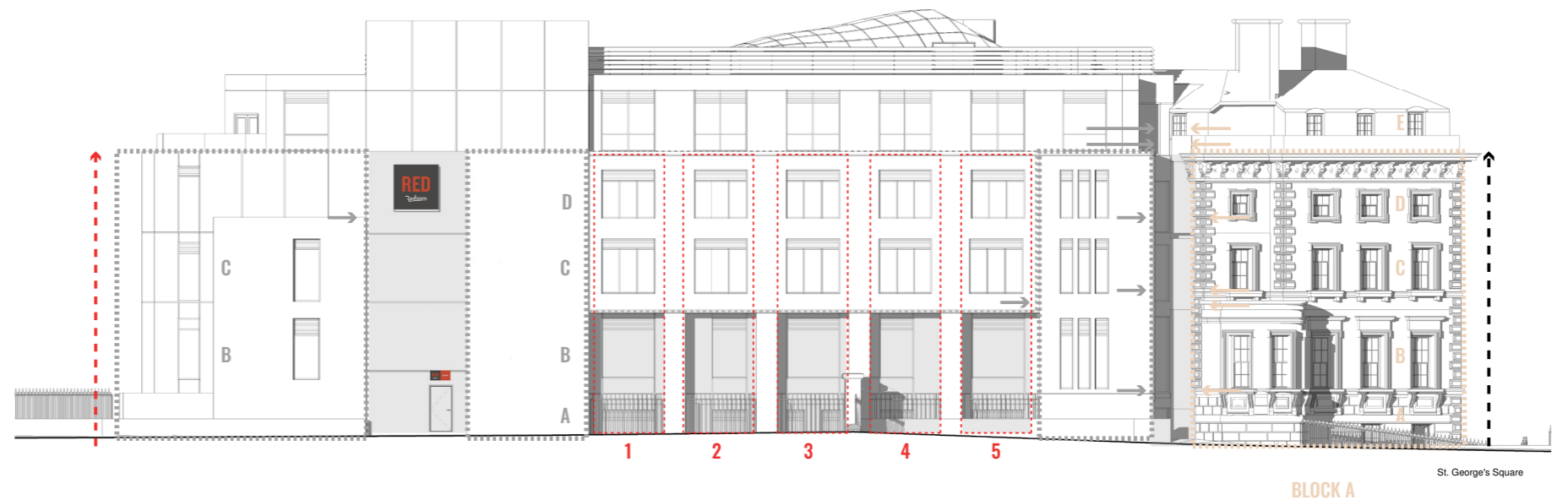
DIAGRAM 8 : West elevation facing from the railway station showing the relationship of the existing architecture and proposed design.
