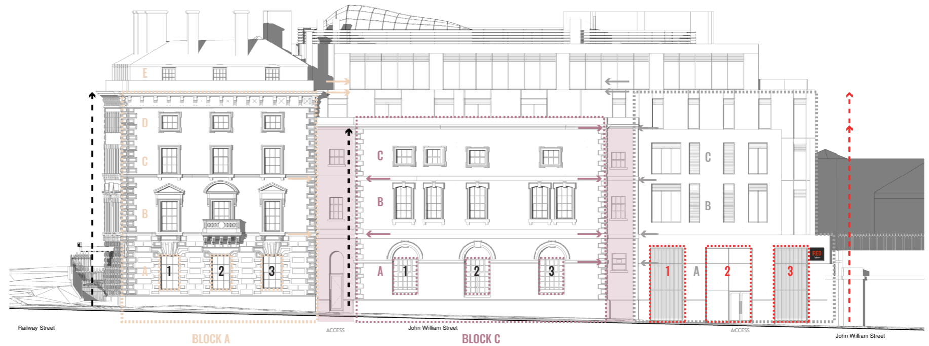
DIAGRAM 7 : John William Street elevation showing the relationship of the existing architecture and proposed design.
