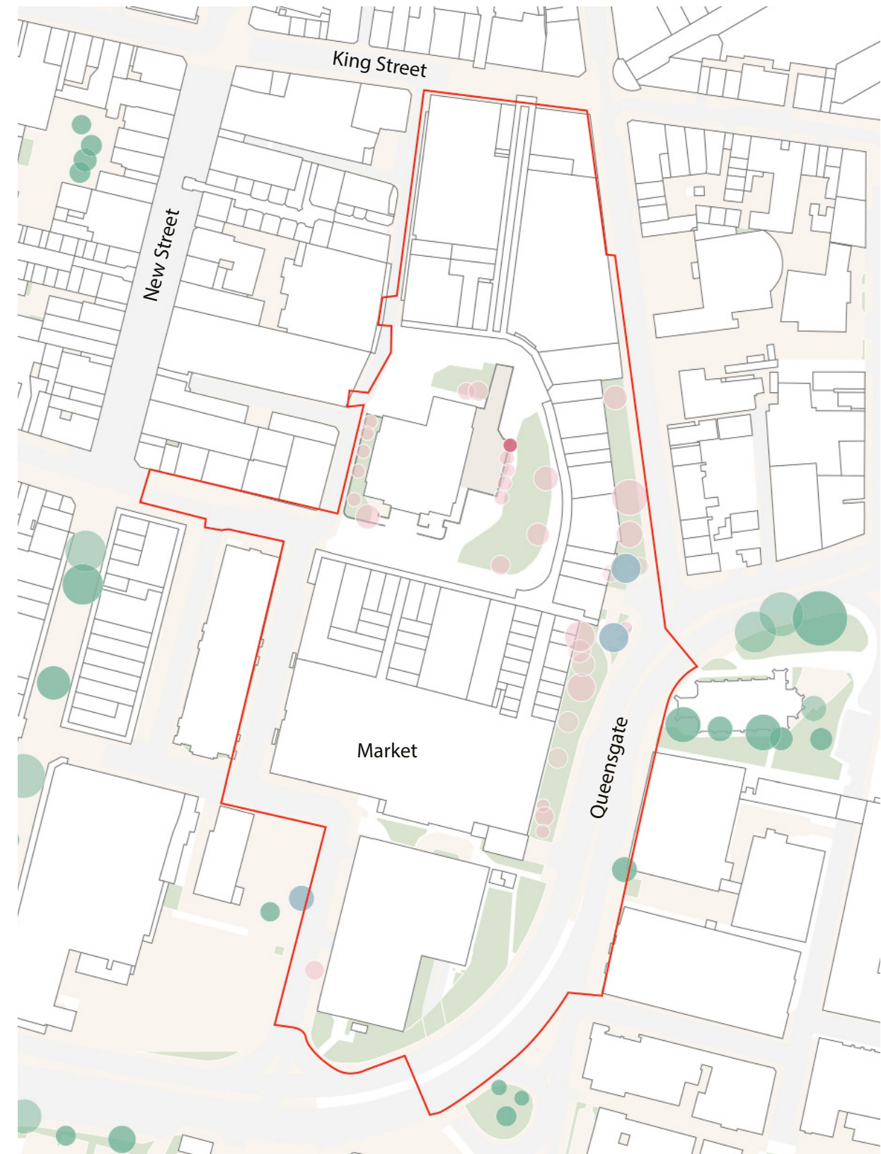
Fig.6.2.1 Existing tree condition plan
