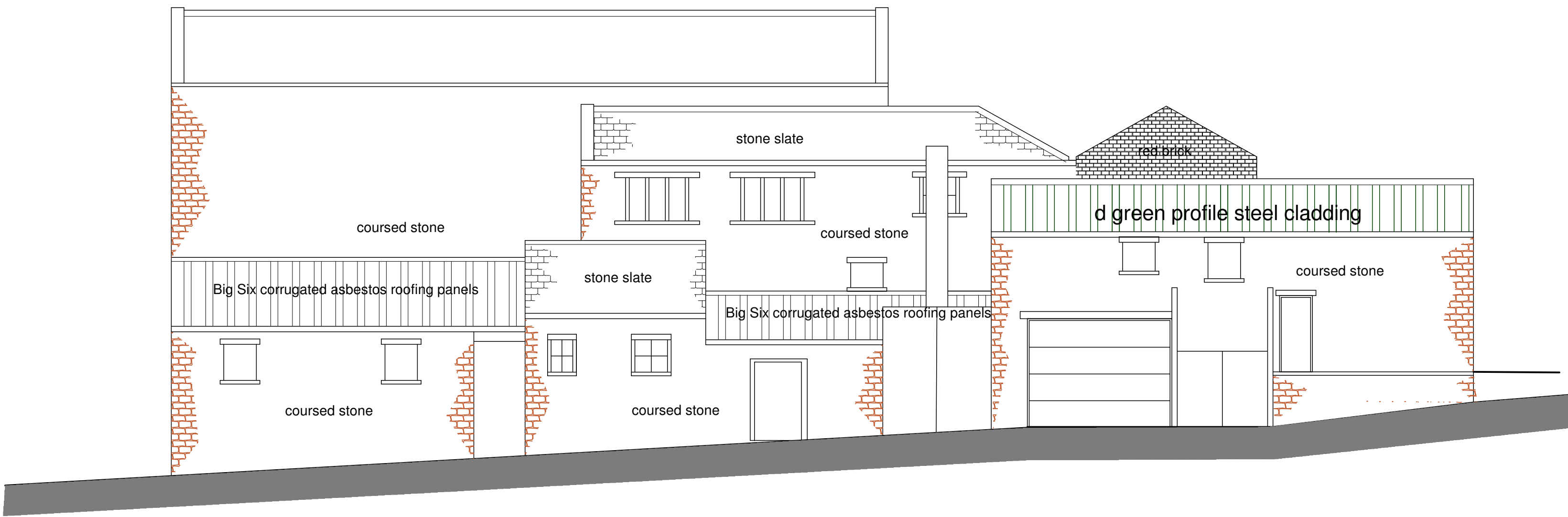
EXISTING NORTH ELEVATION
