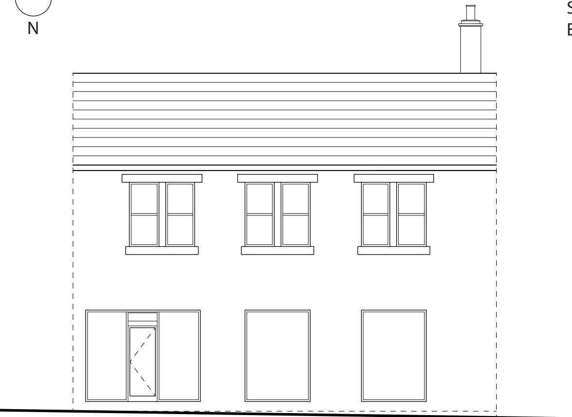
EAST ELEVATION SCALE 1:100 EXISTING - E003
