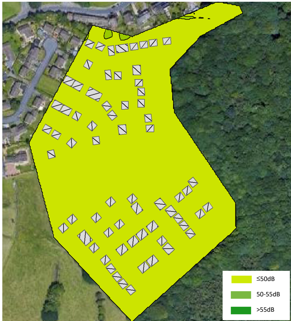
Sound map indicating the external daytime L_{Aeq,16hour} environmental sound levels at head height (1.8m)
