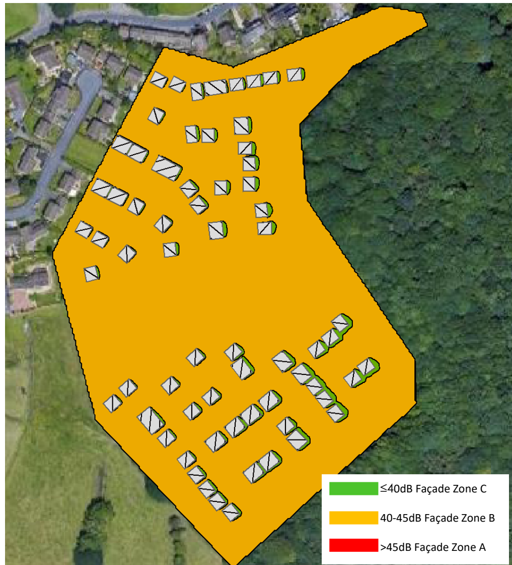
Sound map indicating the external night-time L_{Aeq,8hour} environmental sound levels at 1 st floor level (5.0m)
