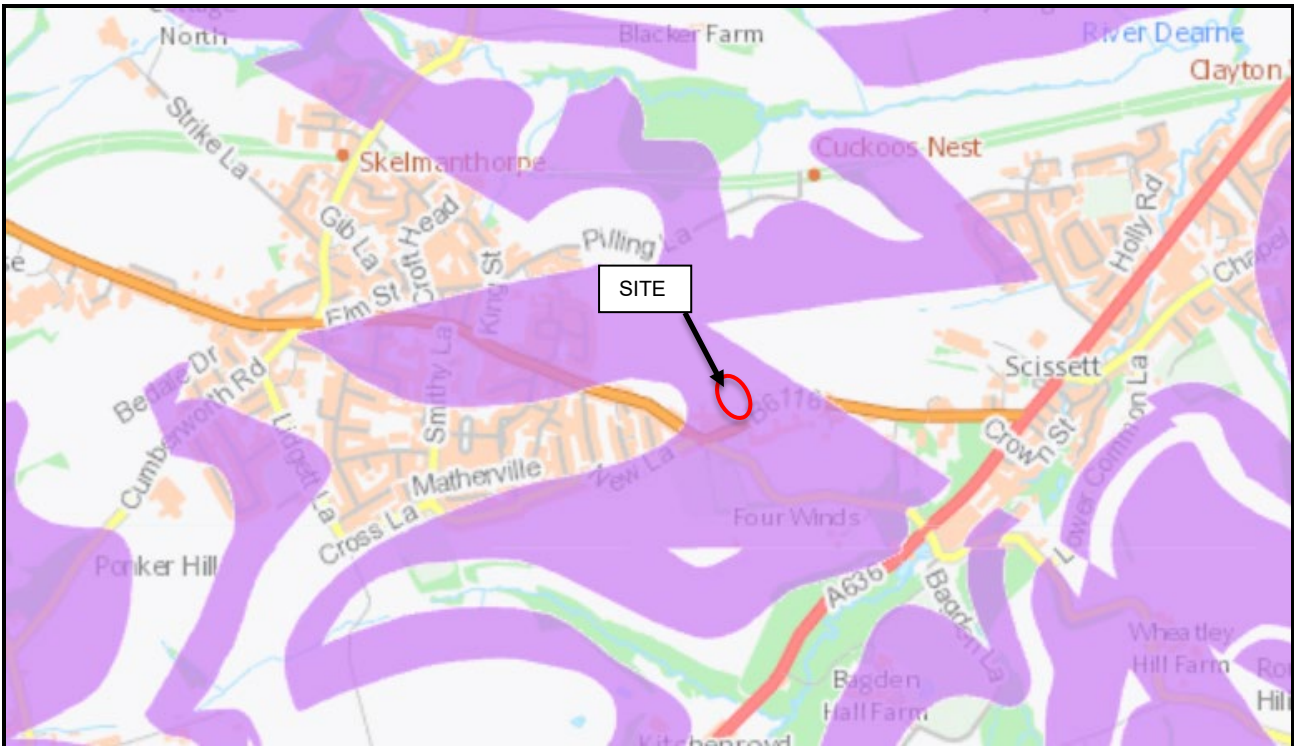
Figure 9 Areas of Probable Shallow Coal Mine Workings
