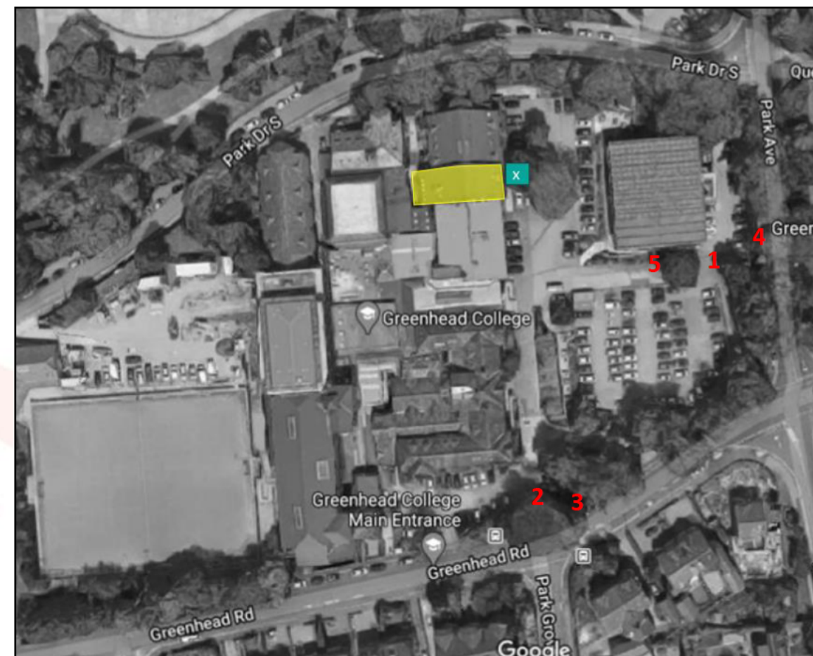
Figure 2: Extract from the DfE provided noise survey report showing the 24-hour measurement location 'X' with Apex Acoustics supplementary short term approximate measurements positions 1 to 5 in red
