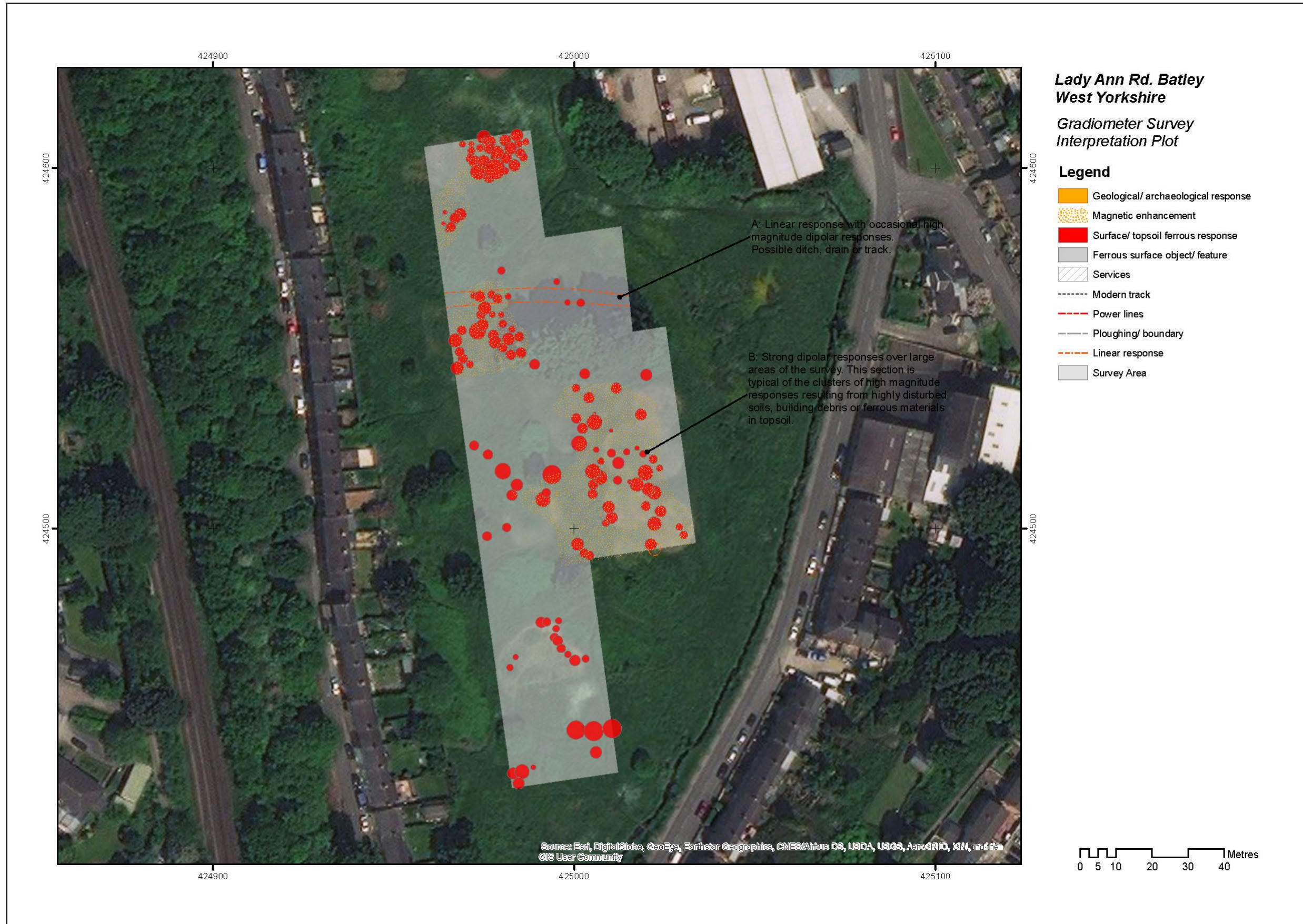
Figure 8. Interpretation with significant anomalies labelled displayed on an aerial photograph of the site
