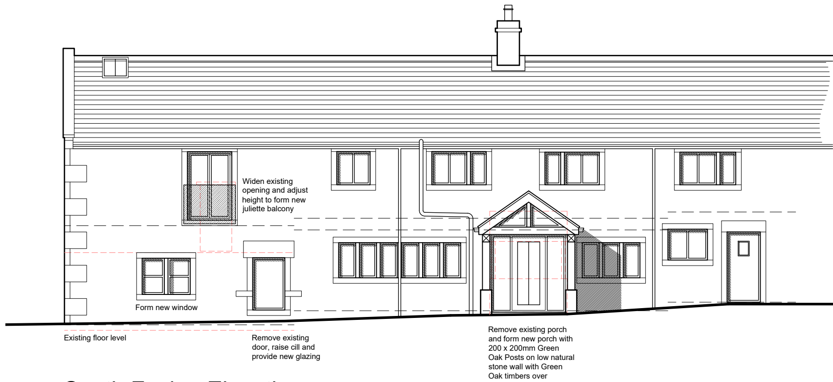
South Facing Elevation
