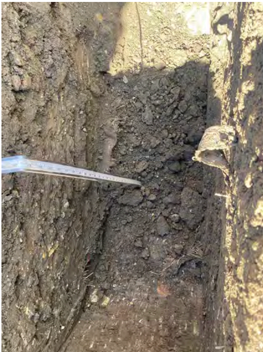
Rear garden of Plot 26 showing 600mm of topsoil
