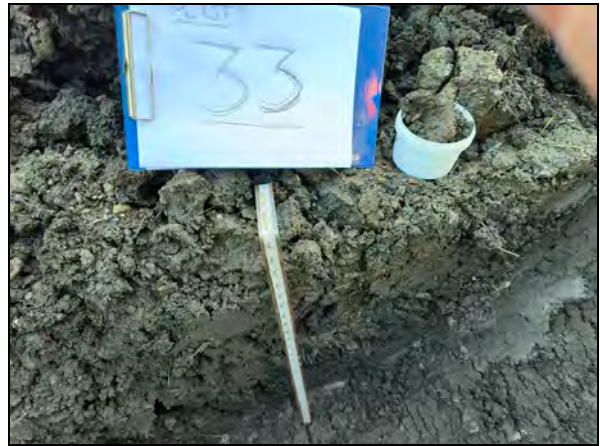
Trial Pits topsoil sampling for Plots 32 and 33, ruler proving depths 600mm
