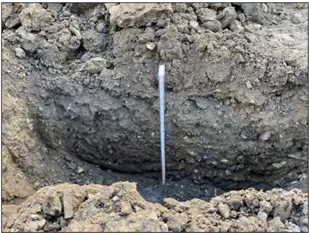
House Plot 30 rear view & Trial Pit proving 600mm of topsoil
