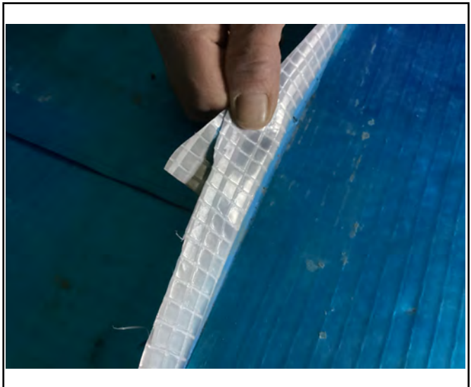
View of the butyl tape identified
