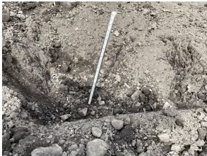
Corner plot of No 22 showing 600mm of topsoil depth
