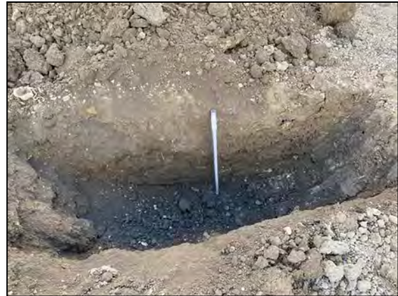
Rear Garden of Plot No 31 showing topsoil proving 600mm depth
