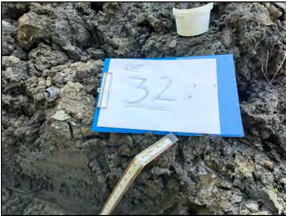
Trial Pits topsoil sampling for Plots 32 and 33, ruler proving depths 600mm
