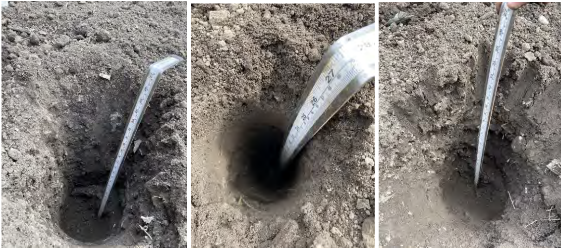
Front garden of Houses 23 – 25 showing 600mm of topsoil
