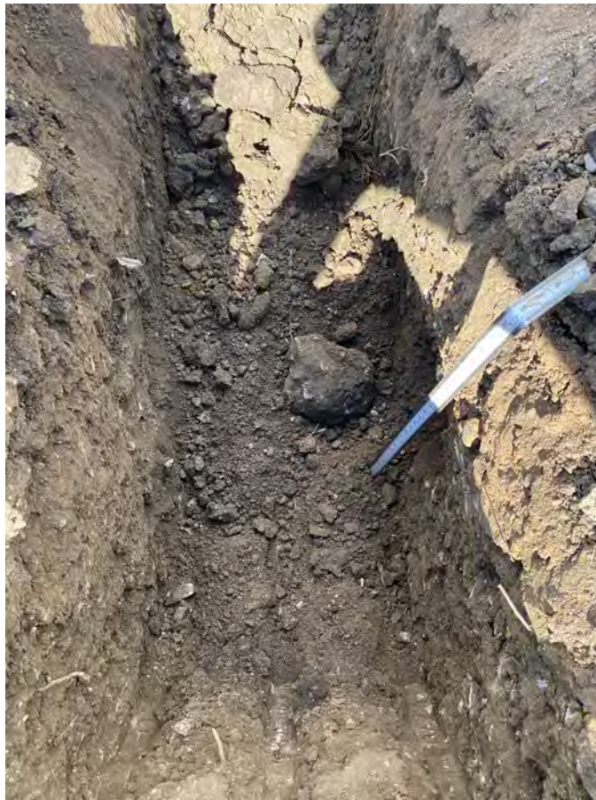
Photo proving 600mm of topsoil in rear garden of Plot 27
