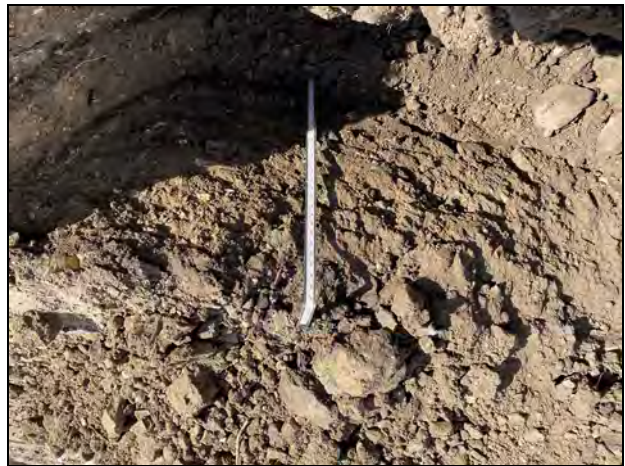
Rear Garden of Plot No 28 showing topsoil proving 600mm depth
