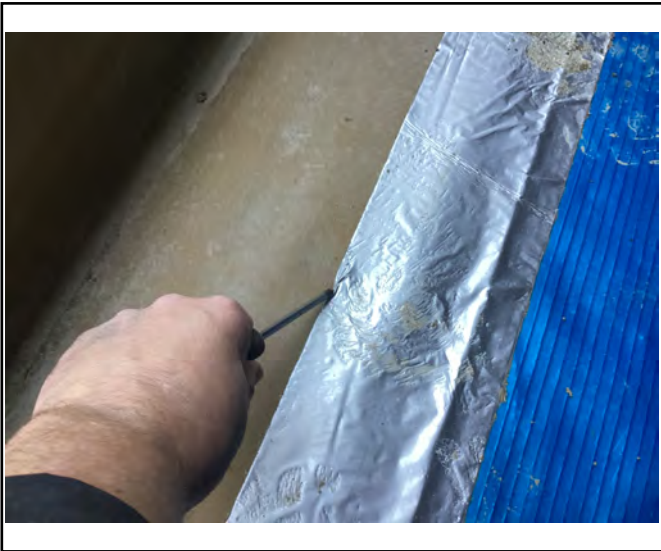
Mechanical Point Stress Test being
