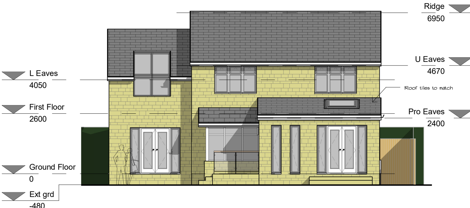
Front Elevation (SW Facing) 1 : 100
