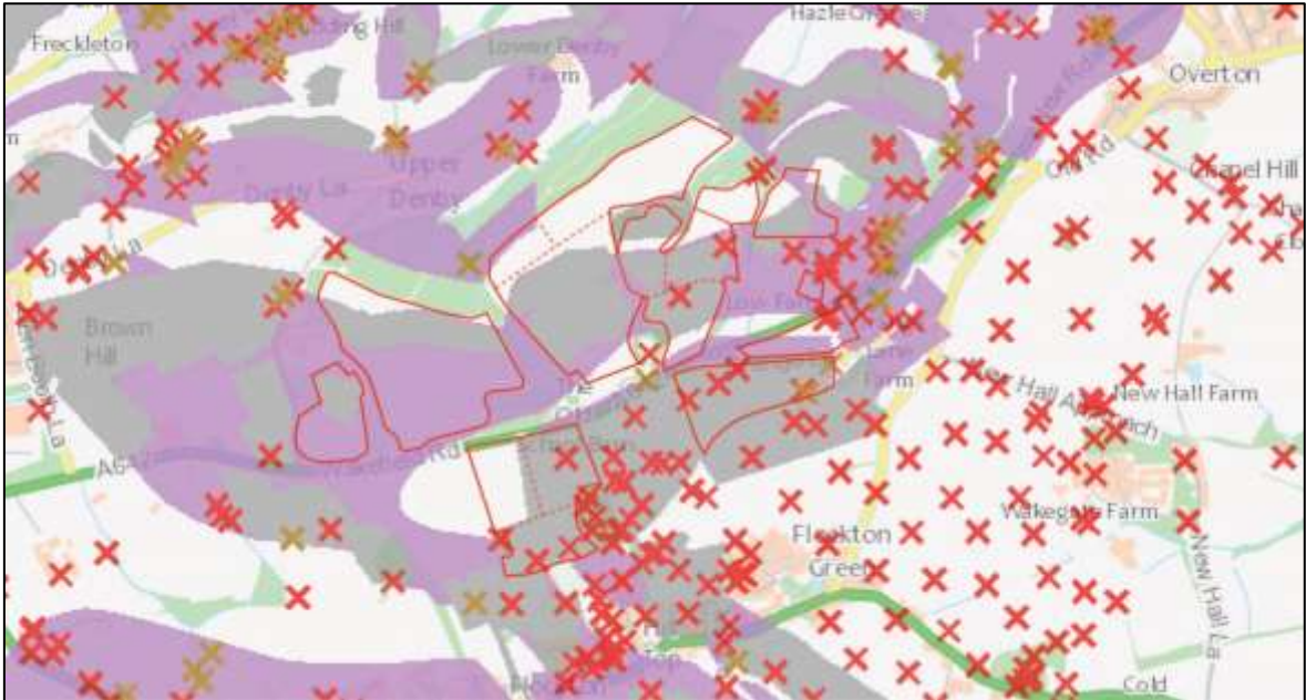
FIGURE 42: IMAGE DERIVED FROM THE COAL AUTHORITY INTERACTIVE VIEWER (SEE REFERENCES). KNOWN SHALLOW WORKINGS IN GREY, AREAS LIKELY TO HAVE BEEN SUBJECT TO SHALLOW WORKING IN PURPLE; MINE ENTRY MARKED AS RED (SHAFT) OR BROWN (ADIT) CROSSES. THE SITE IS INDICATED.
