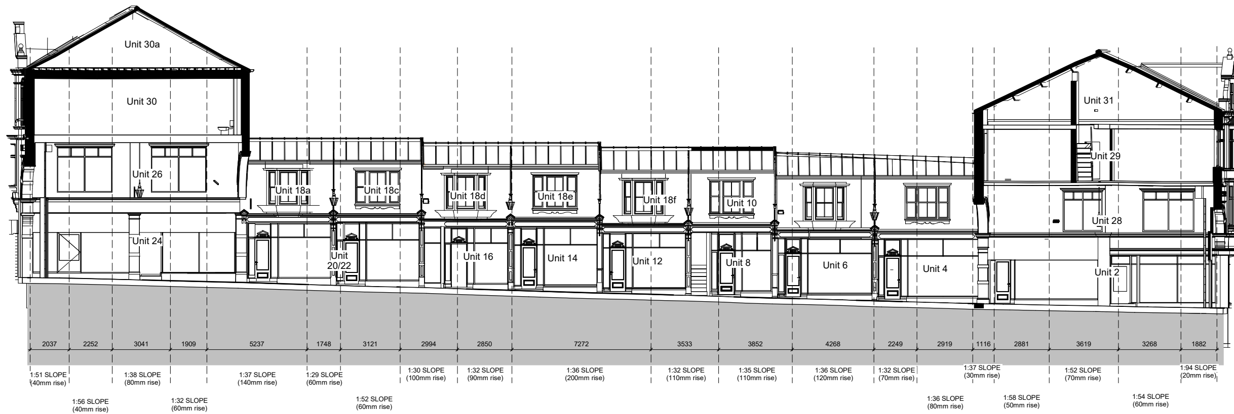
Figure 5.3.5 Existing slope gradients
