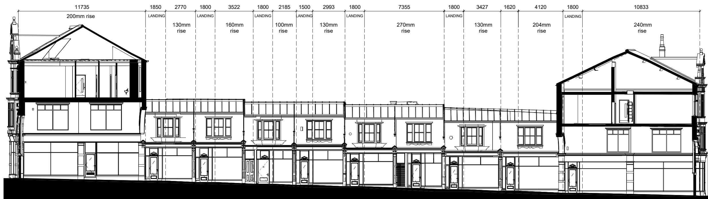
Figure 5.3.8 New slope gradients
