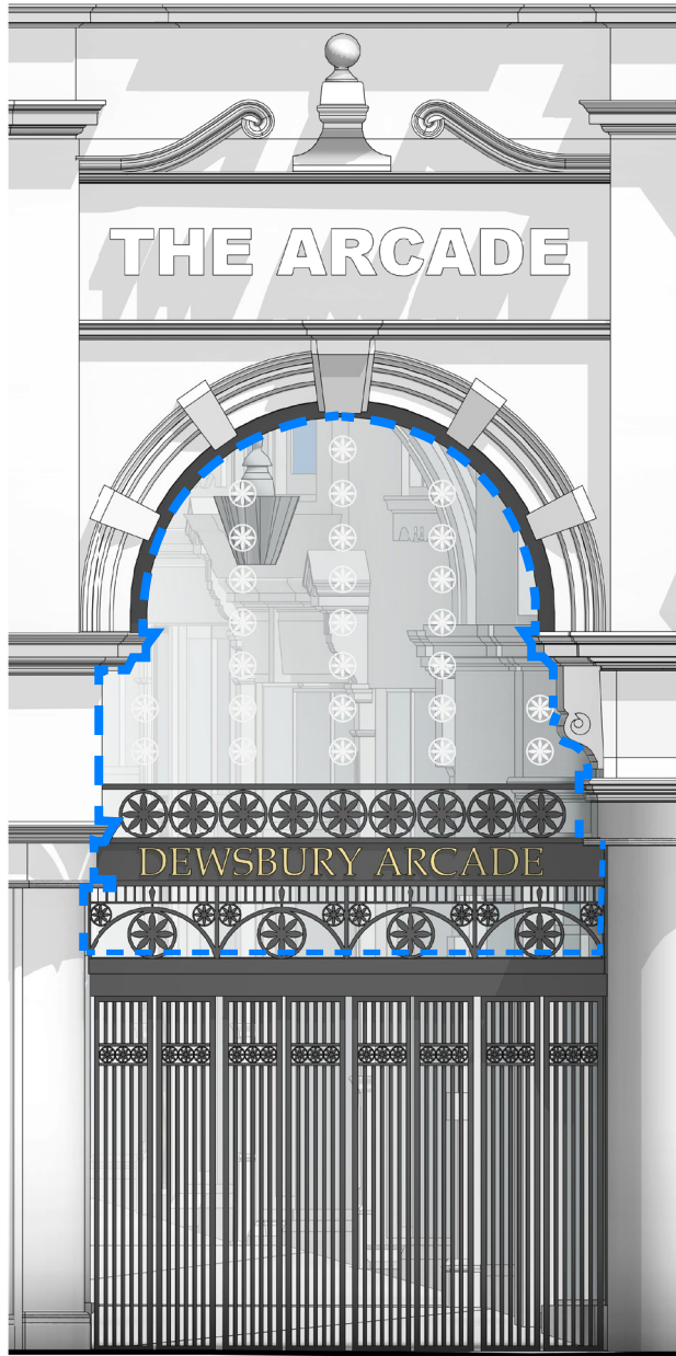
Figure 4.5.3 Entrance gate glazing
