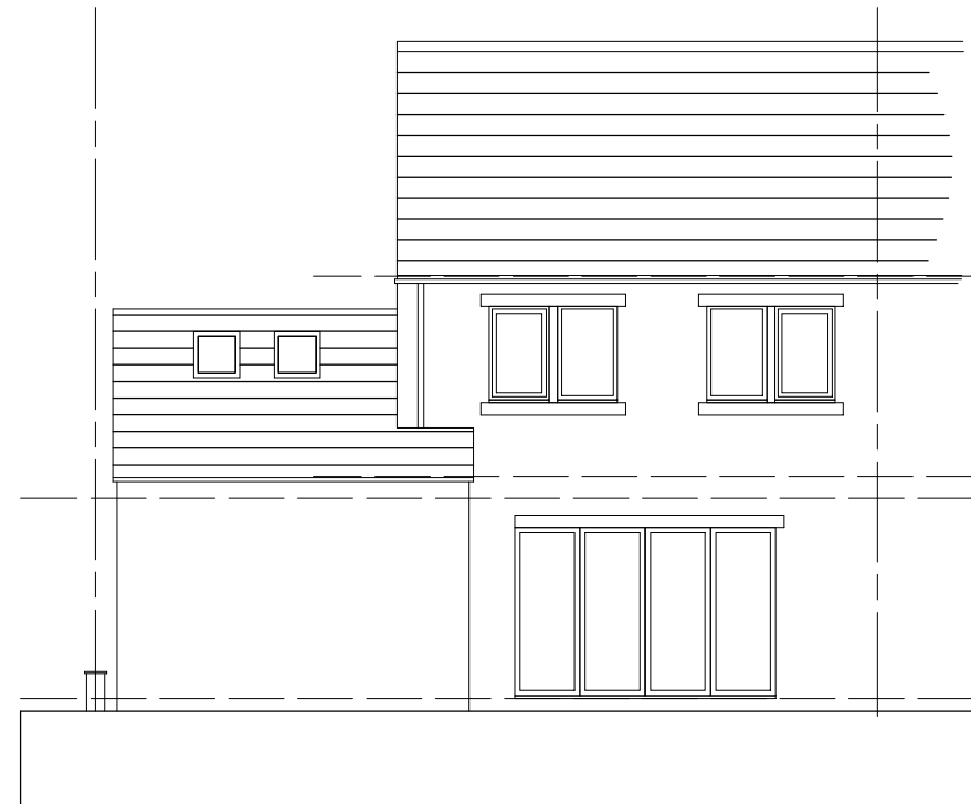
REAR ELEVATION_ AS PROPOSED Scale 1.100
