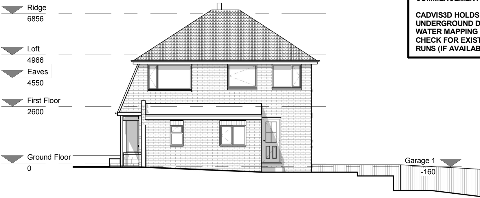
Side Elevation (North Facing) 1 : 100
