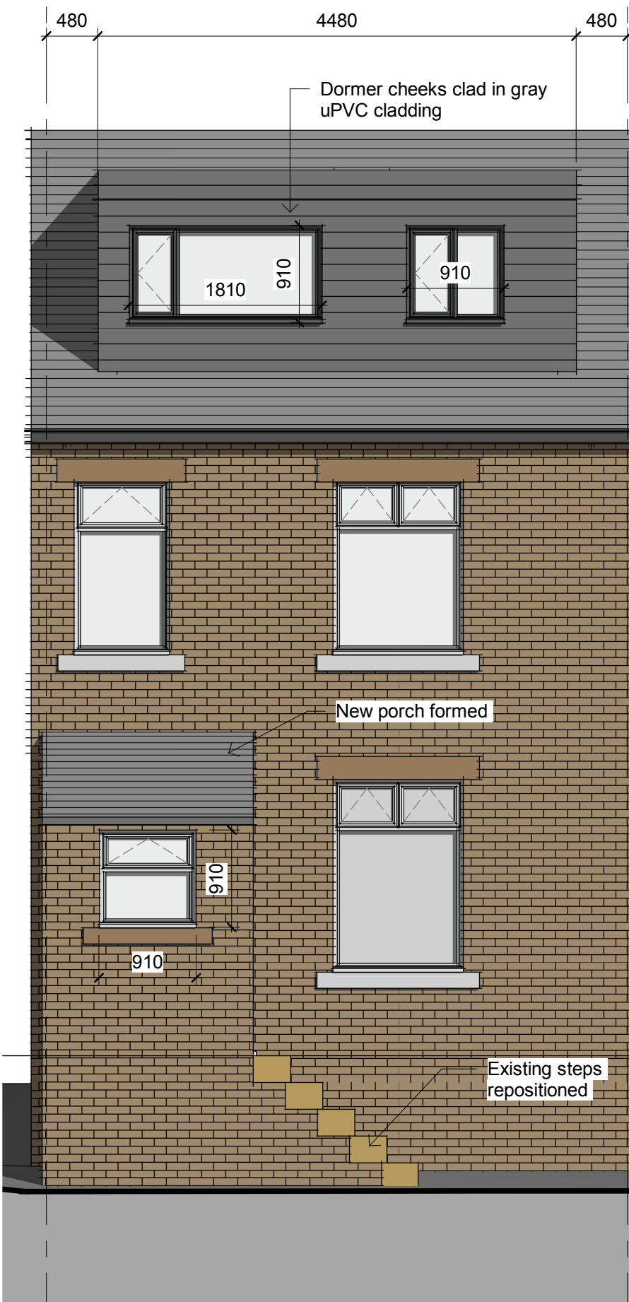
Proposed Rear Elevation 1 : 50
