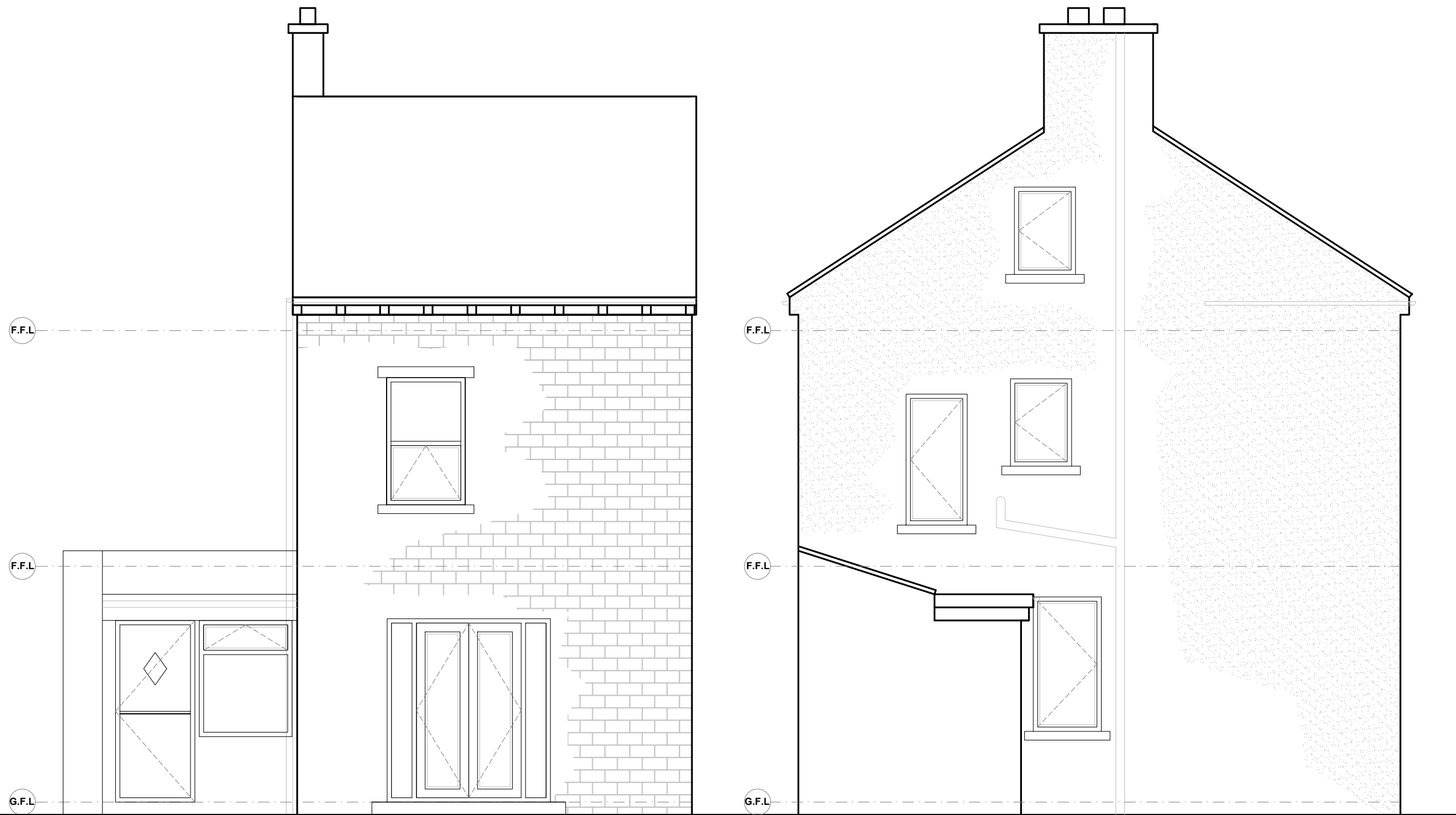
EXISTING FRONT ELEVATION SCALE 1:50
