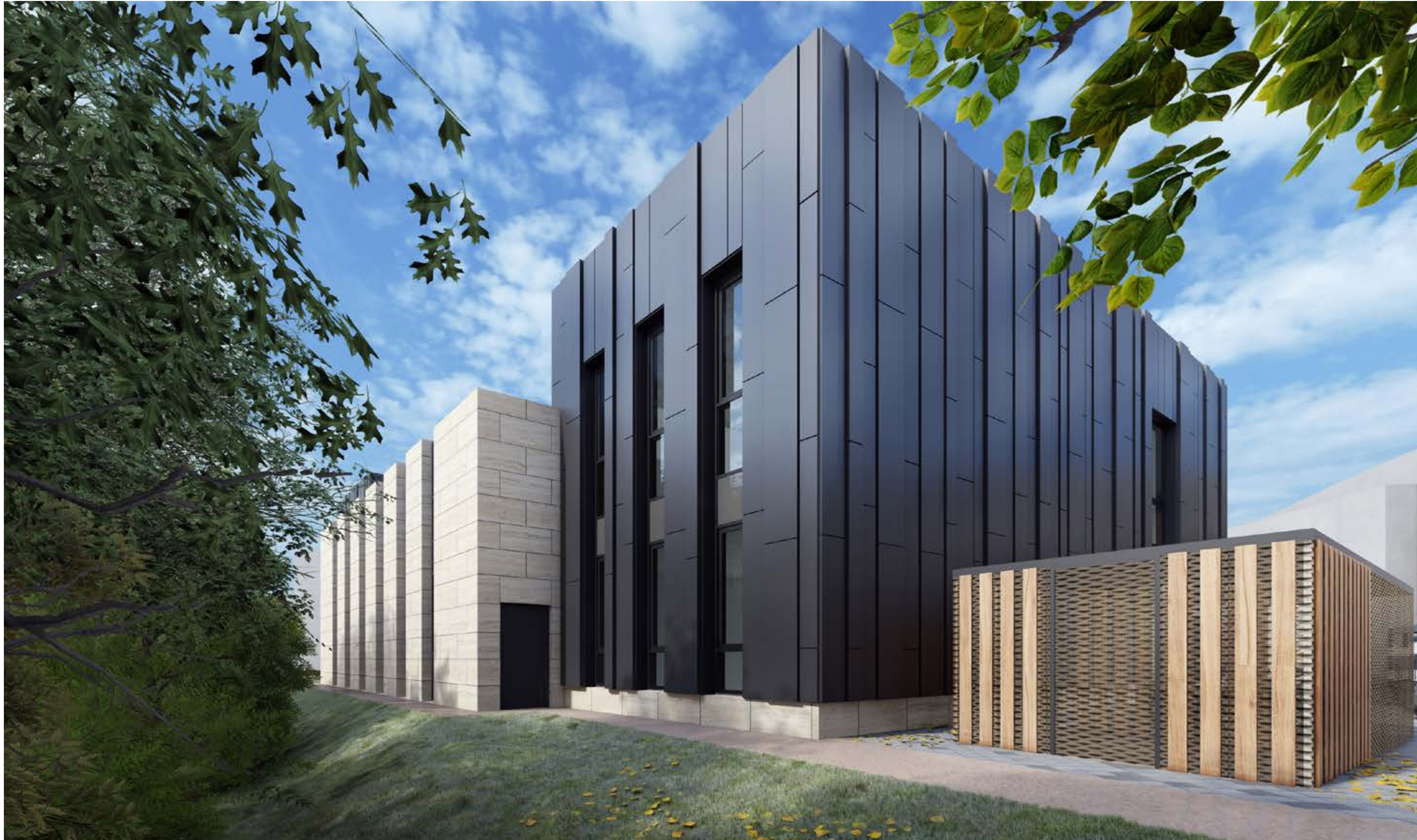
View from the Huddersfield Narrow Canal. The Congregation Hall is expressed externally by dropping the roof level and wrapping the Ashlar stone plinth up and around it.
