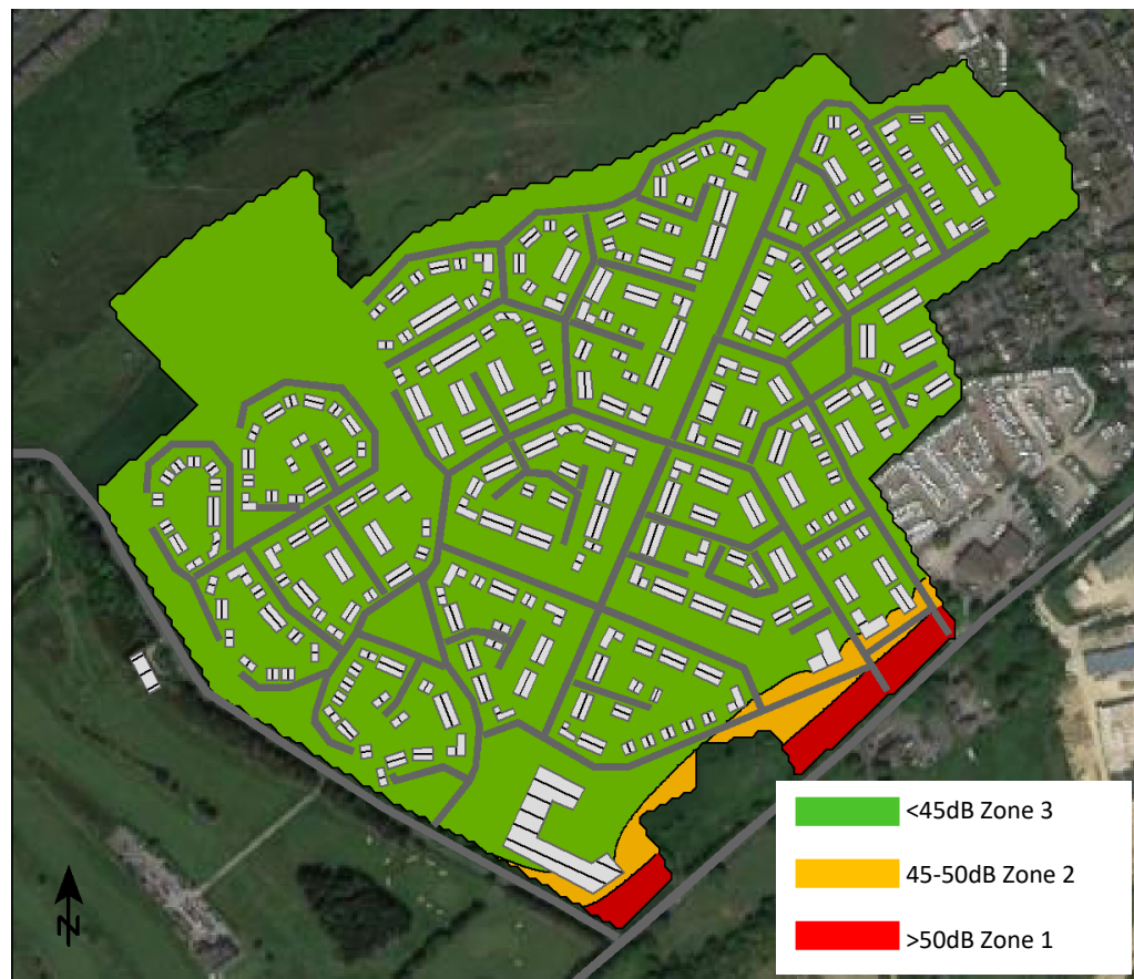
Sound map indicating the external night-time L_{Aeq,8hour} environmental sound levels at 1 st floor level (5.0m)
