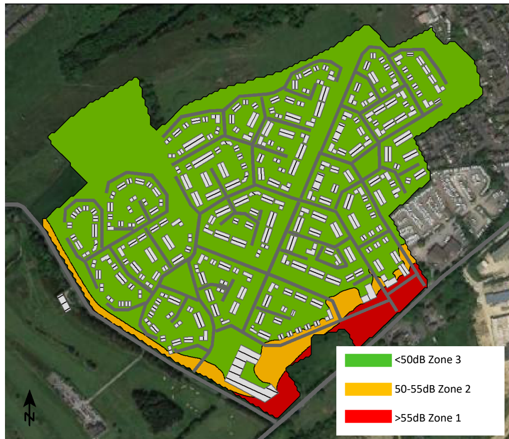
Sound map indicating the external daytime L_{Aeq,16hour} environmental sound levels at Ground floor level (2.5m)
