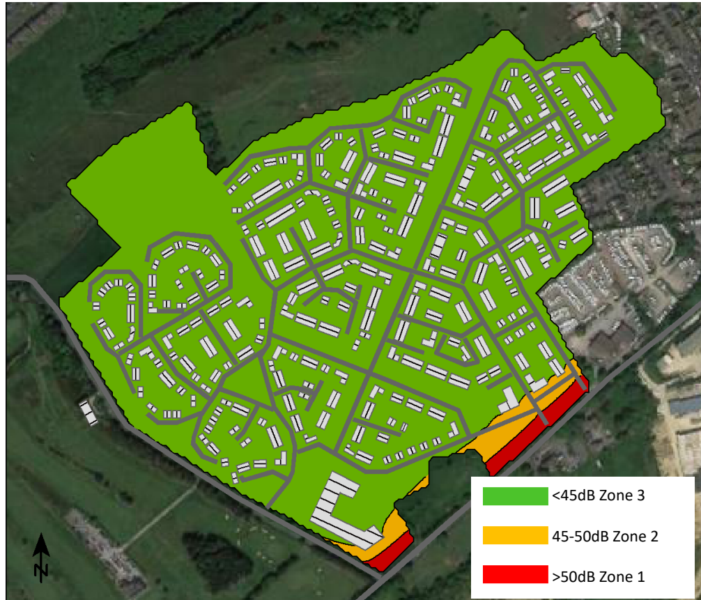
Sound map indicating the external night-time L_{Aeq,8hour} environmental sound levels at Ground floor level (2.5m)
