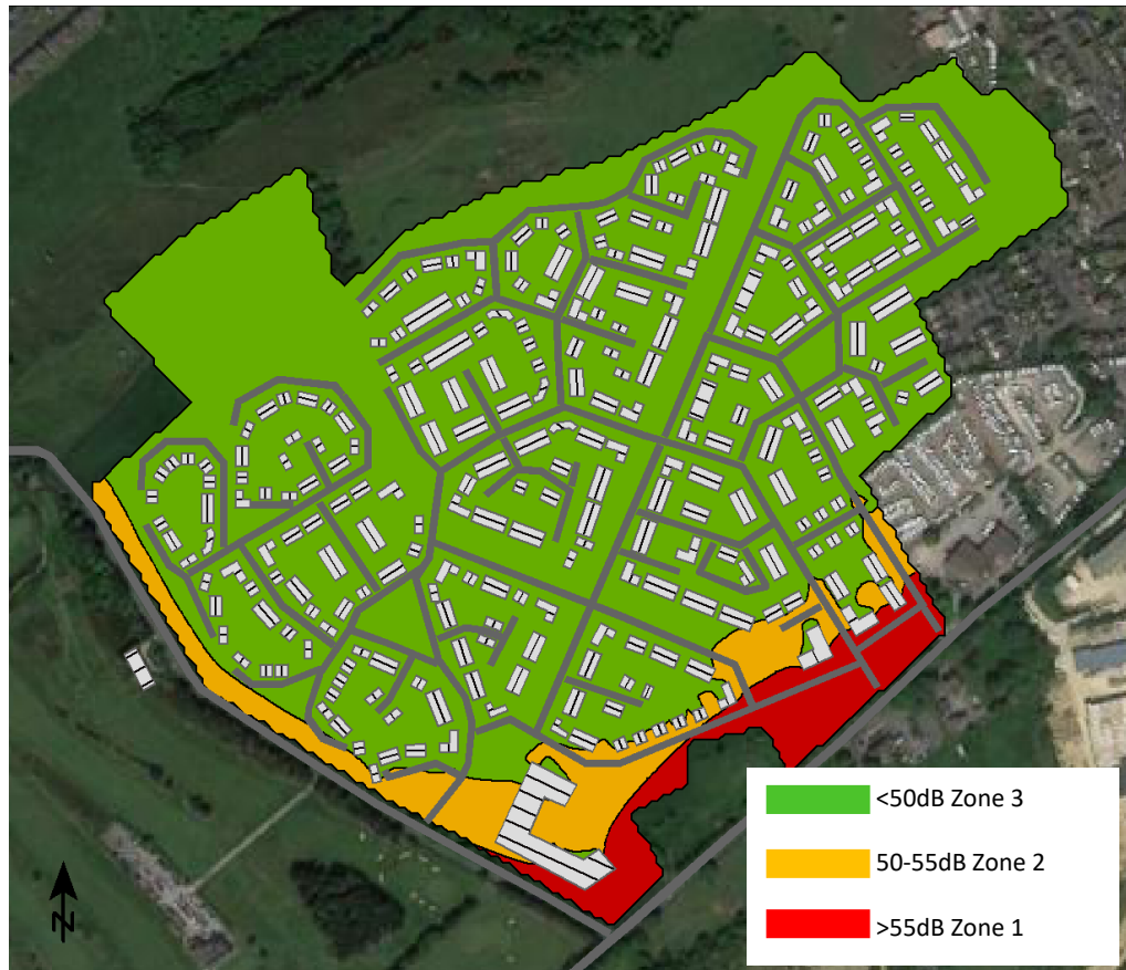
Sound map indicating the external daytime L_{Aeq,16hour} environmental sound levels at 1 st floor level (5.0m)
