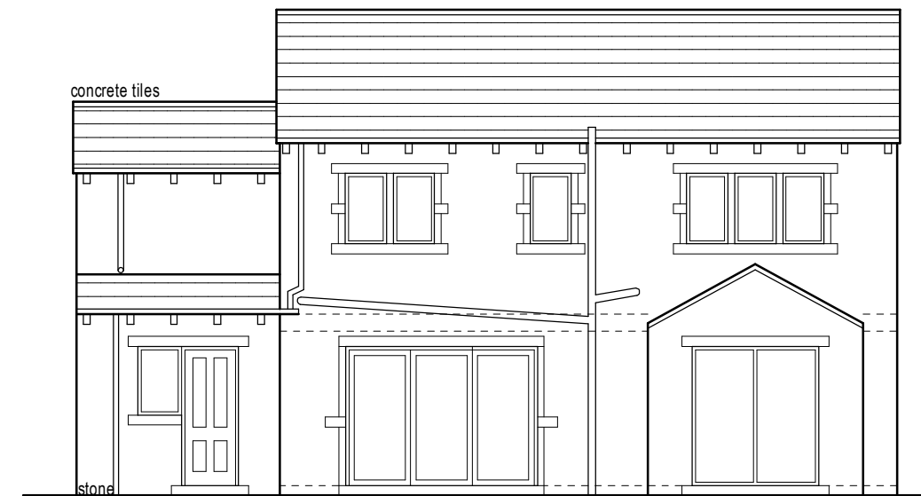
Existing rear elevation (1:100)
