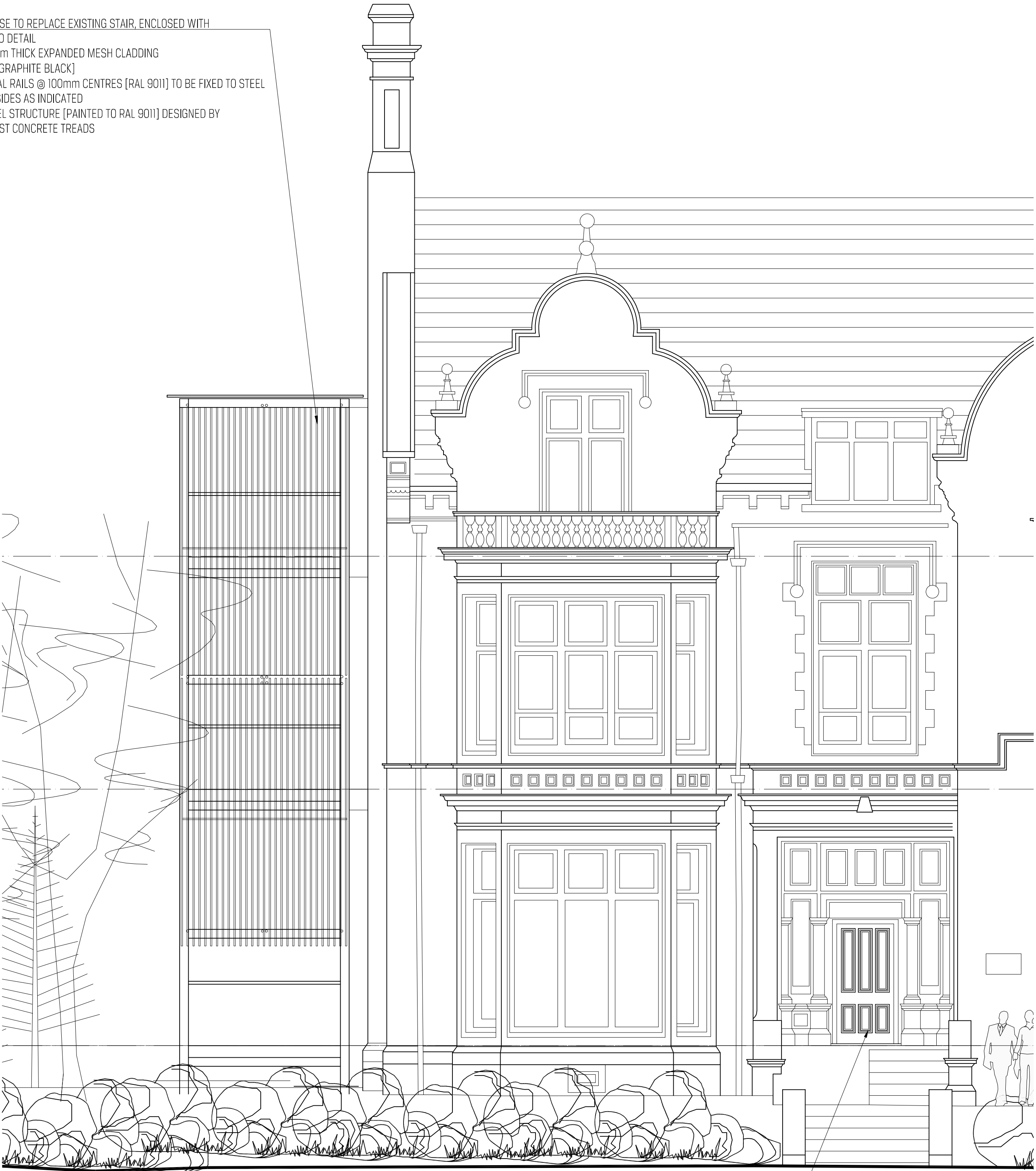
EXTERNAL STAIRCASE SOUTH ELEVATION | SCALE 1:50
