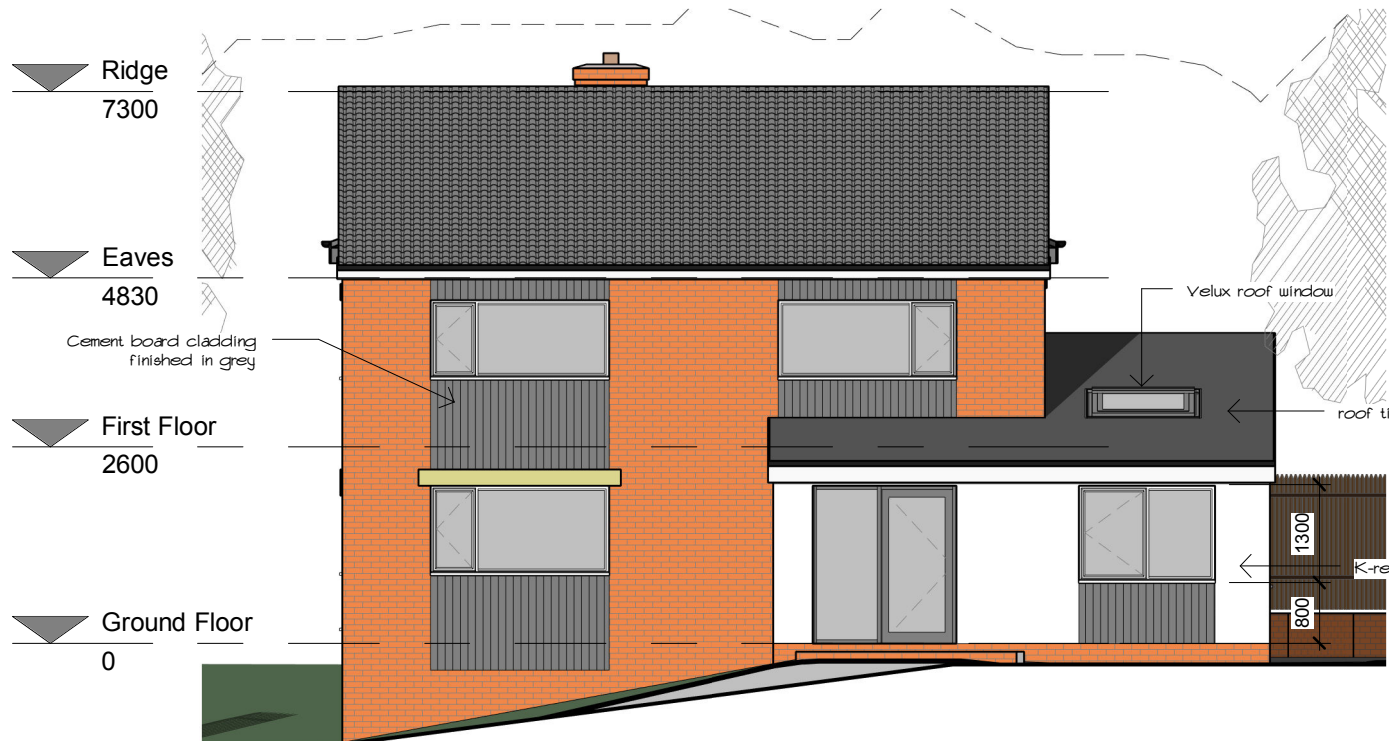
Front Elevation (East Facing) 1 : 100
