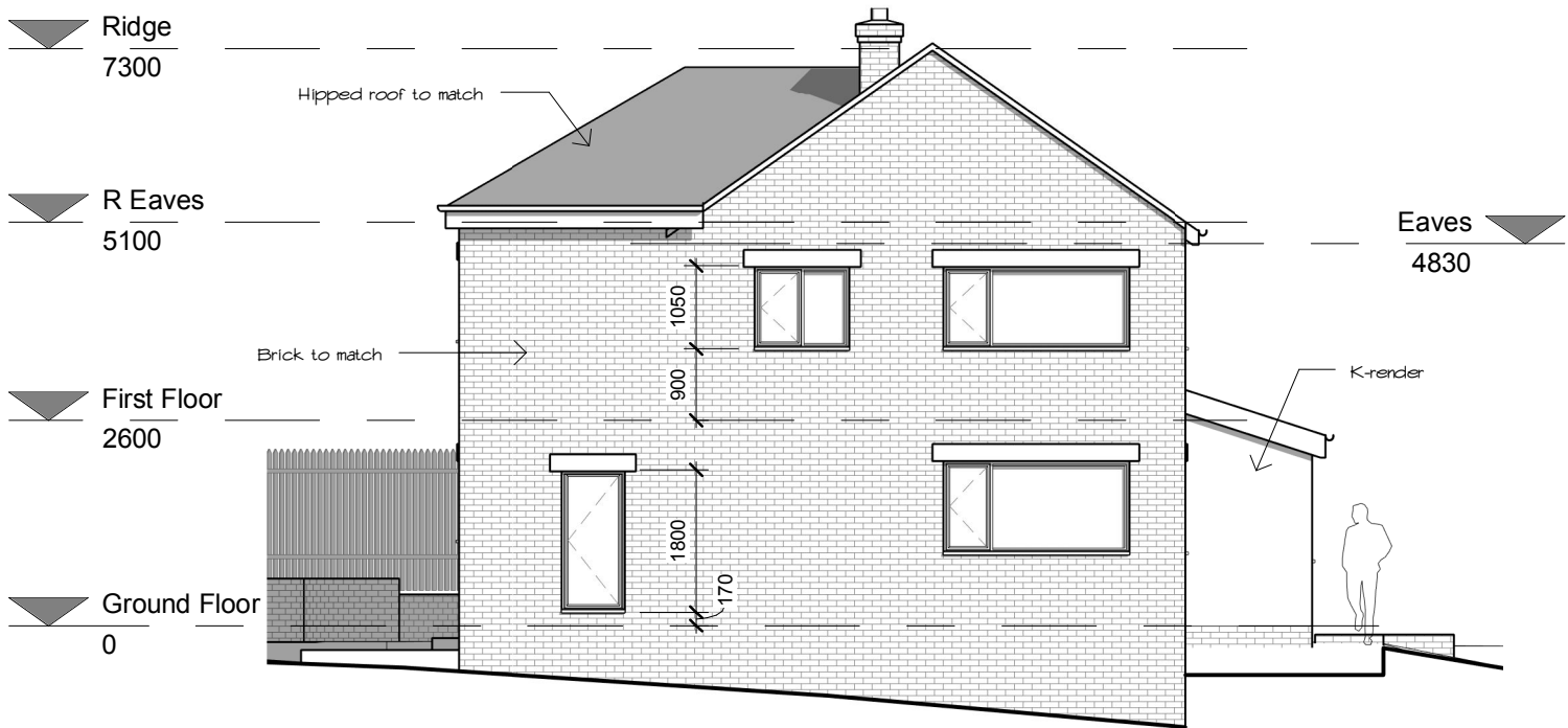
Side Elevation (South Facing) 1 : 100
