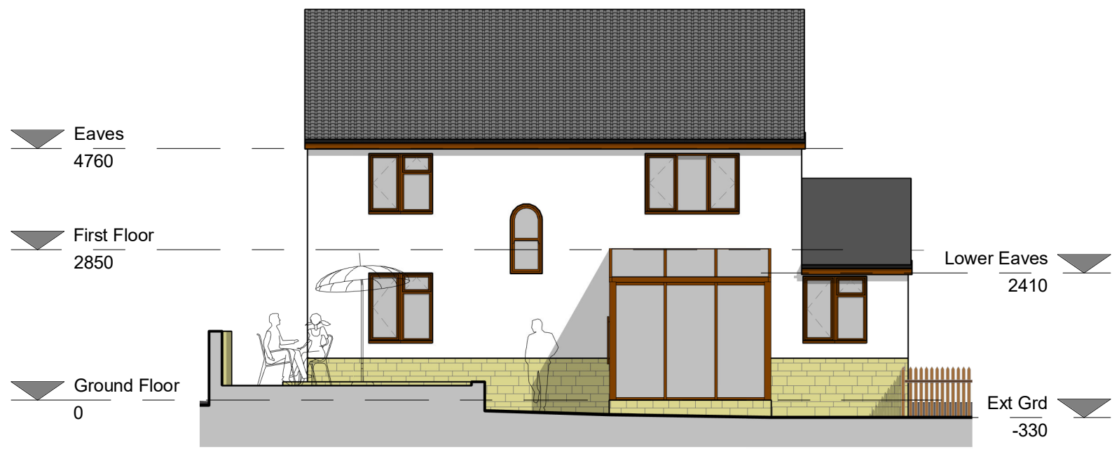
Rear Elevation (South Facing) 1 : 100
