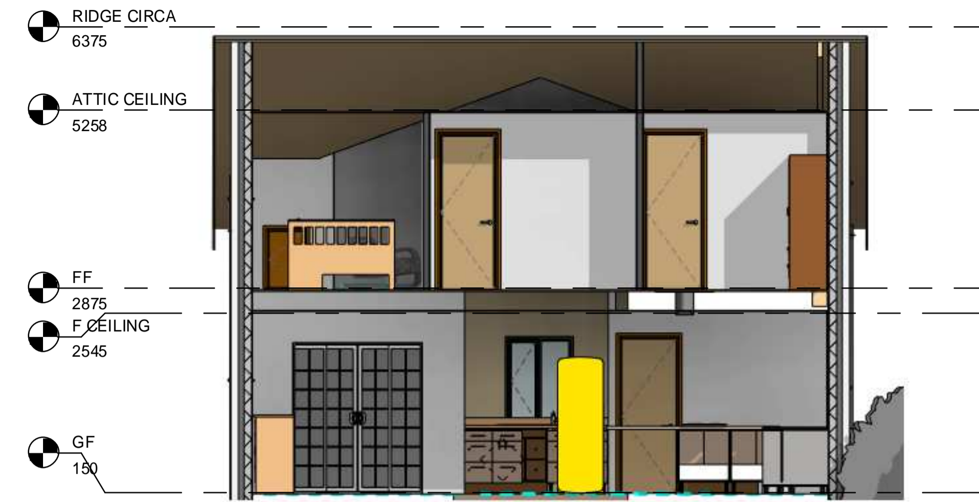
6 SECTION THRU CENTRE OF BUILDING 1 : 50
