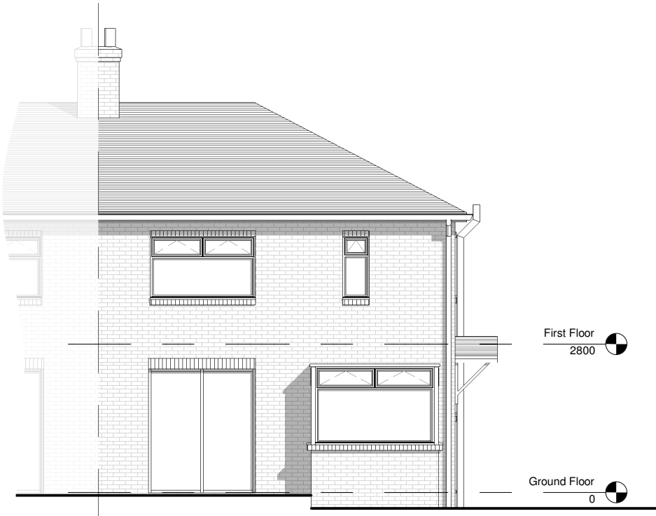
South Elevation - Existing 1 : 100
