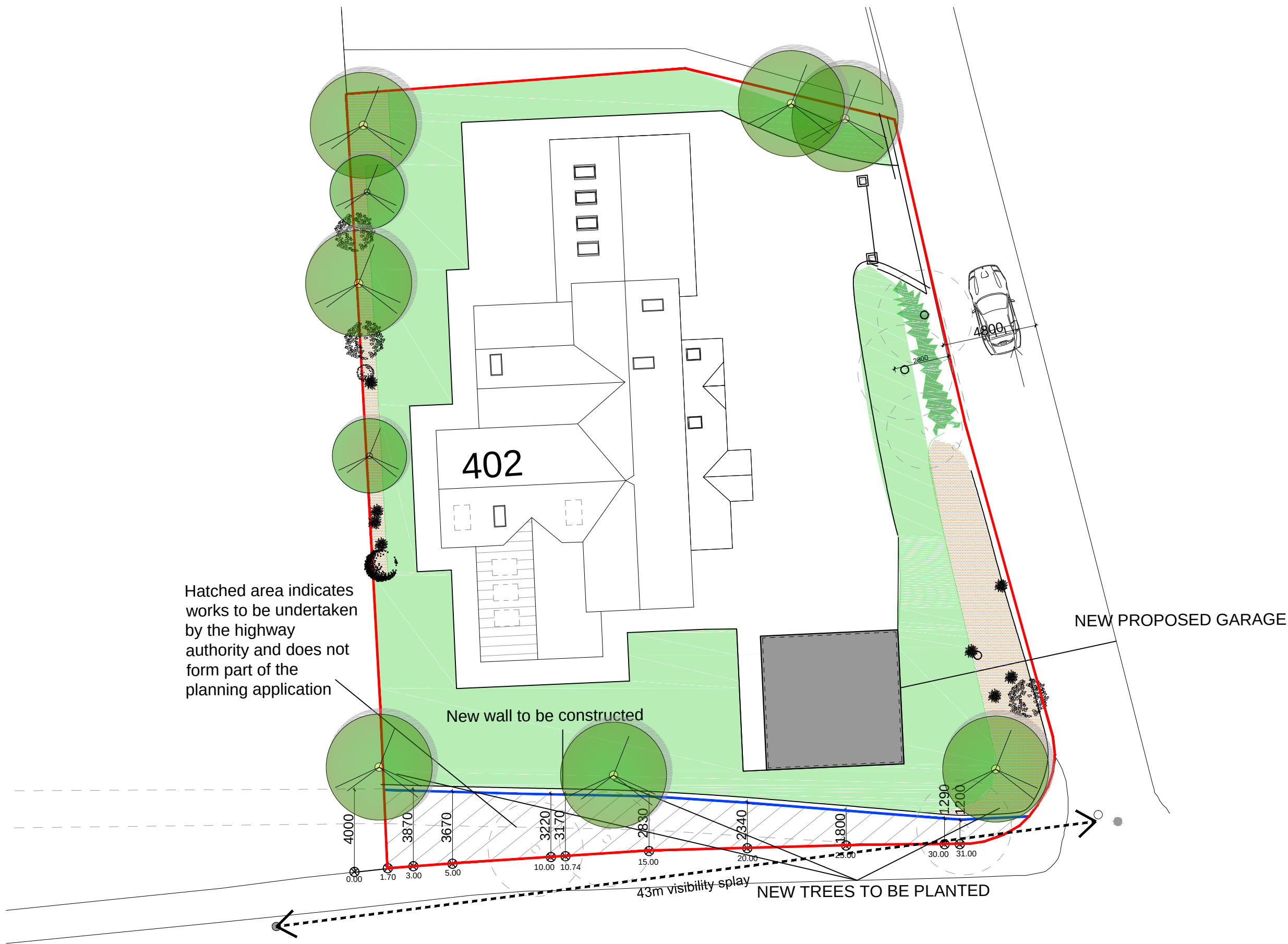
PROPOSED SITE PLAN 1:200 AFTER JUNCTION IMPROVEMENT WORKS 1:200
