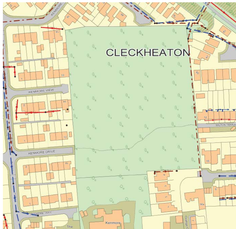
Figure 5 – NWL Sewer Network
