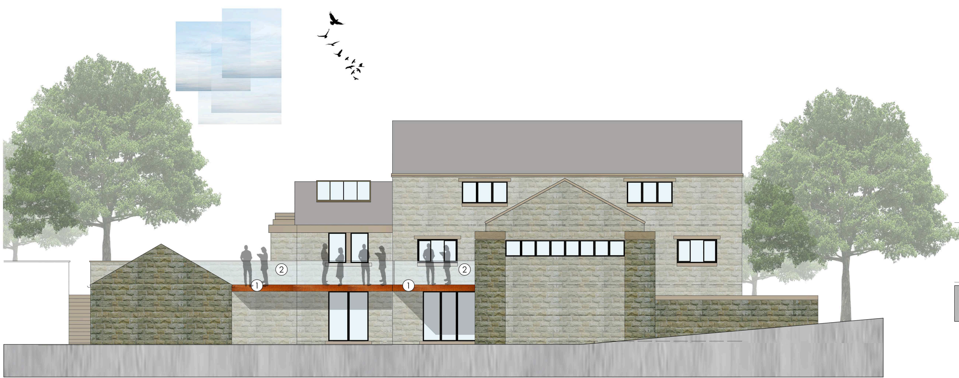
FRONT CONTEXT ELEVATION AS PROPOSED_ Scale 1_100
