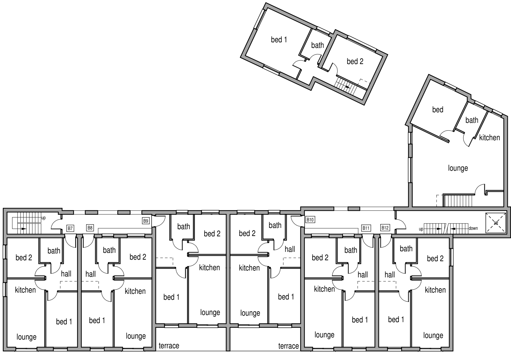
Proposed buildings B and C first floor layout (1:200).
