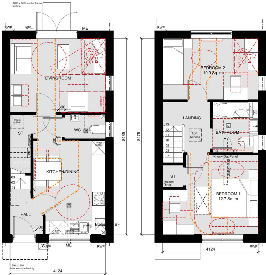
Ground Floor Plan Area to blockwork - 35.6m 2 (384ft 2 ) Area to plasterboard - 35.0m 2 (377ft 2 )
