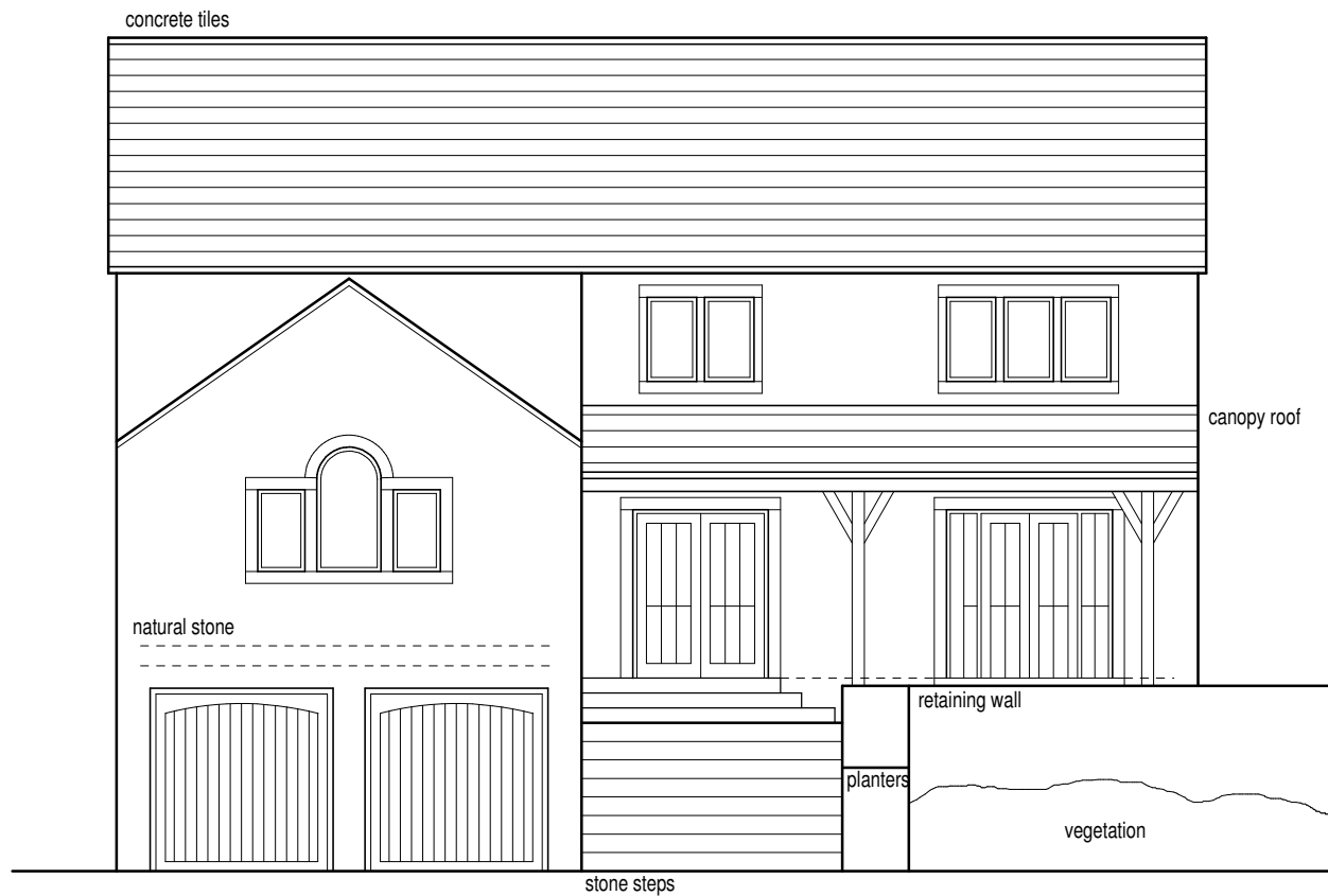
Existing front elevation (1:100)
