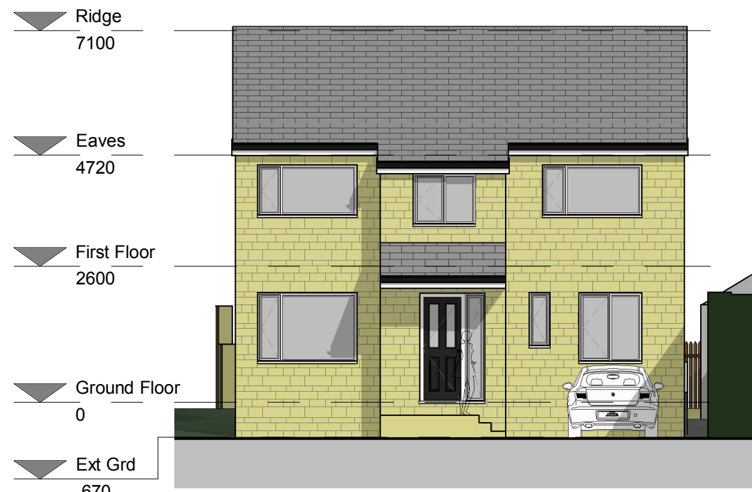
Front Elevation (North Facing) 1 : 100
