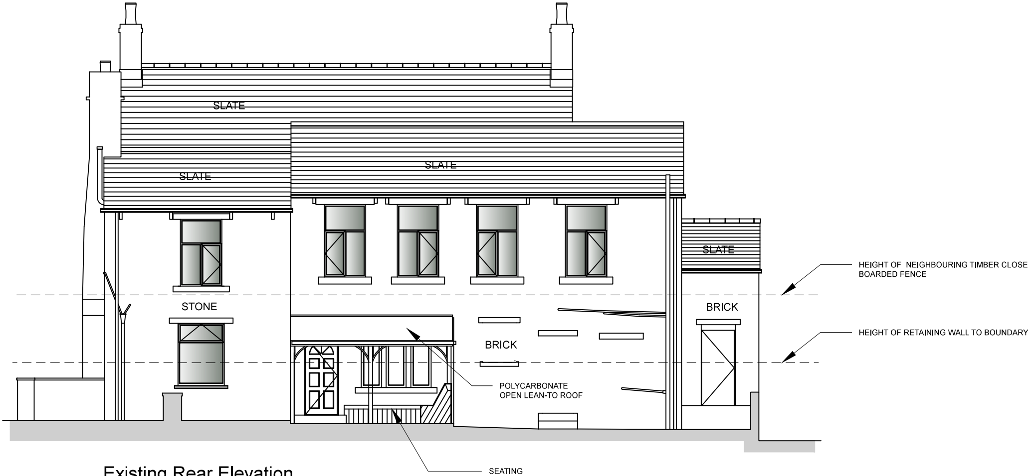
Existing Rear Elevation
