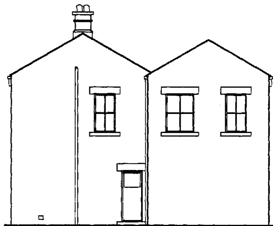
PROPOSED SIDE ELEVATION (SOUTH WEST) - SCALE 1:100
