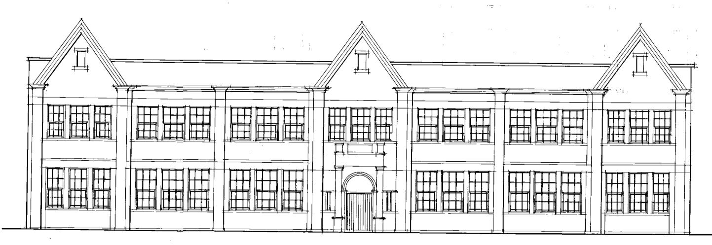
EXISTING FACADE TO REMAIN. ALL STONE REPAIRS TO BE CARRIED OUT AS REQUIRED EXISTING WINDOW OPENINGS TO BE FITTED WITH NEW PAINTED HARDWOOD WINDOWS
